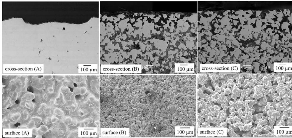
Fig. 2. SEM of the cross-section and top surface of Fe-2wt%P parts sintered at 1100 °C: (A) in resistive furnace, (B) in Ar plasma and (C) in H<sub>2</sub> plasma.
