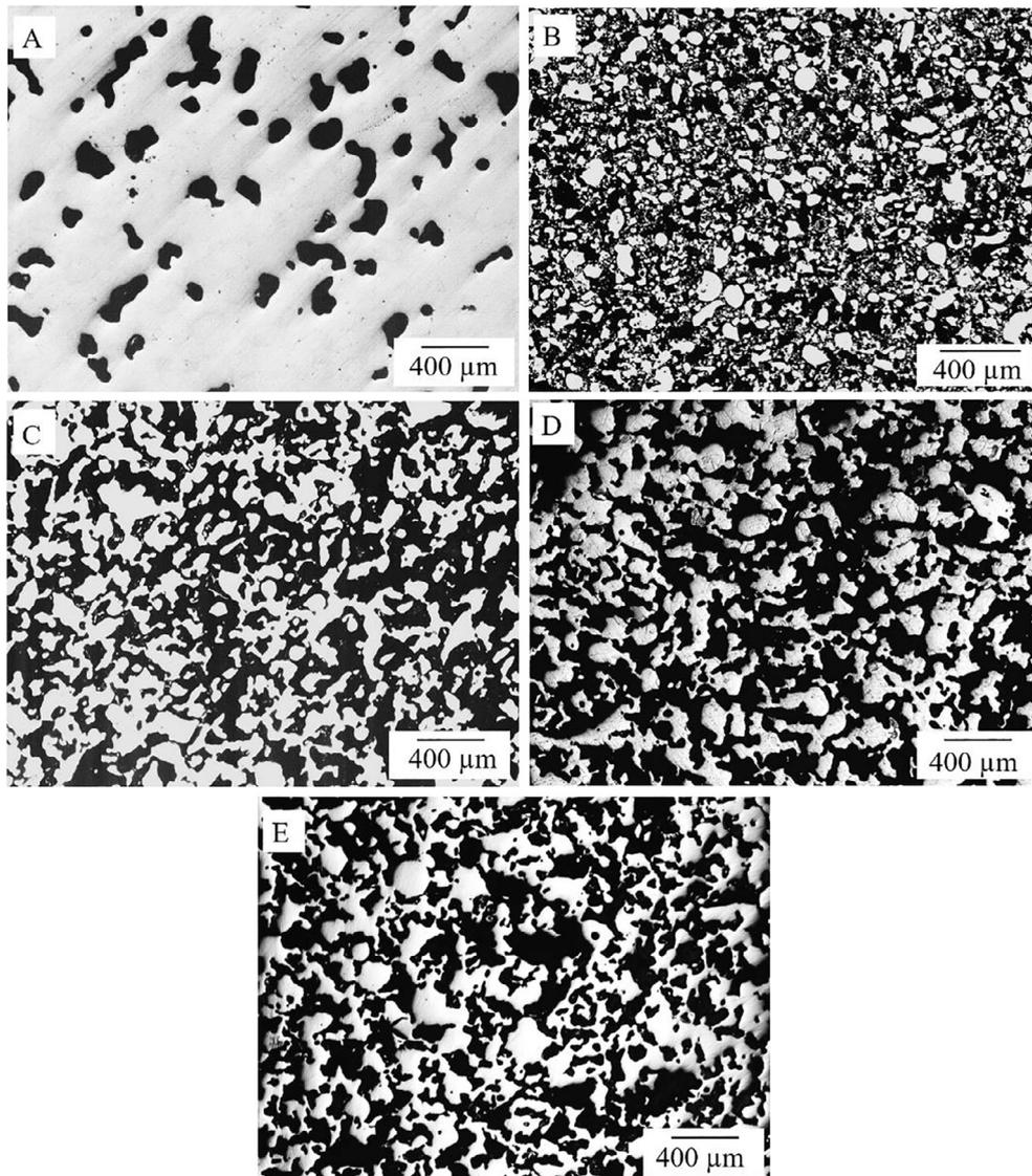
**Fig. 1.** Microstructure of injection-molded parts produced with 50 vol% of Fe-2%P and sintered in: (A) resistive furnace at 1100 °C, (B) Ar plasma at 900 °C, (C) Ar plasma at 1100 °C, (d) H<sub>2</sub> plasma at 1100 °C and (E) injection-molded part produced with 53 vol% of Fe-2%P and sintered in Ar plasma at 1100 °C.
