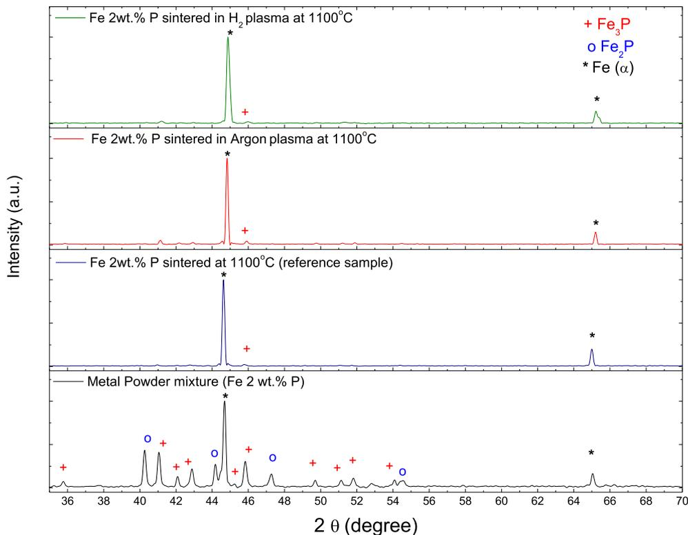
Fig. 3. X-ray pattern of injection-molded parts regarding sintering parameters.
